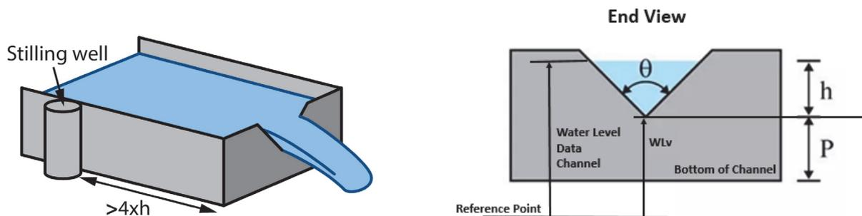
The HOBOLink water flow calculations for a v-notch weir assume the following:
