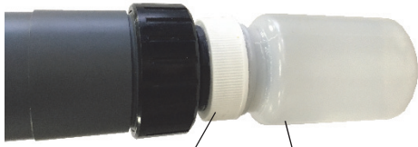
First, slide on storage solution cap Then, insert sensor end cap in the bottle
