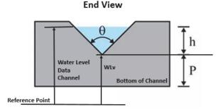
The HOBOlink water flow calculations for a v-notch weir assume the following:
