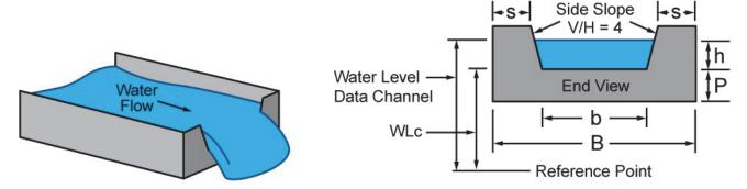
The HOBOlink water flow calculations for a trapezoidal weir assume the following:
